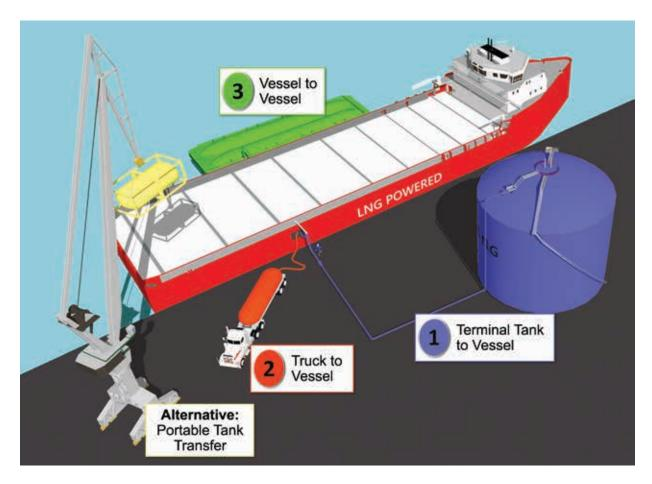
Figure 4. Standard LNG Bunkering Options
