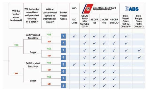
Figure 8. Bunker Vessel Decision Tree
