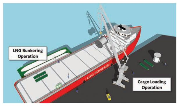
Figure 12. Example SIMOPS: LNG Bunkering and Cargo Loading
